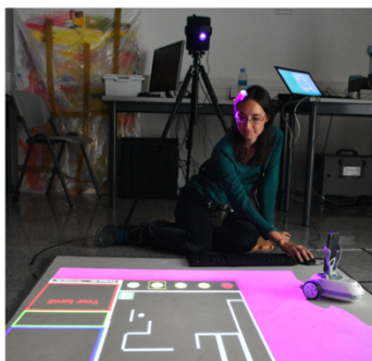
Figure 39: Maze testbed setting where a user is playing with the robot.
