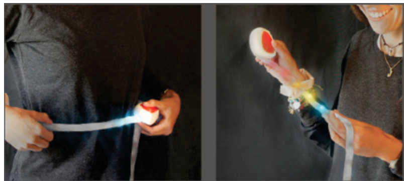
Figure 32: An example of the LED measuring tape showing the progression for the user.
